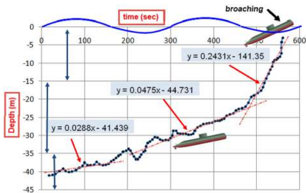
Fig. 12. Depth change due to the suction force from surface waves. Initial depth: 40 m, speed: 5 knots, regular waves height: 2.5 m, period: 8 sec, wave length: 103 m
