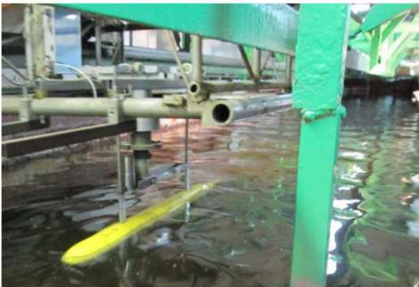
Fig. 3. Persia-110 model in the marine laboratory of the Admiral Makarov National University of Shipbuilding
